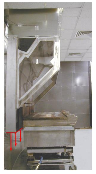
Two Charbroilers, Simulated Cooking -- C&C 3500 cfm Exhaust 2000 cfm MUA (57%) through Rear Discharge
