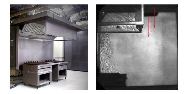
Performance similar to the back supply when velocities are minimized by maximizing perforated area
