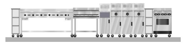
per IMC for Heavy Duty Equipment:18 ft. x 400 cfm/ft.=7200 cfmper UMC for high temperature :18 ft x 4 ft x 100 cfm/ft<sup>2</sup> =7200 cfm
